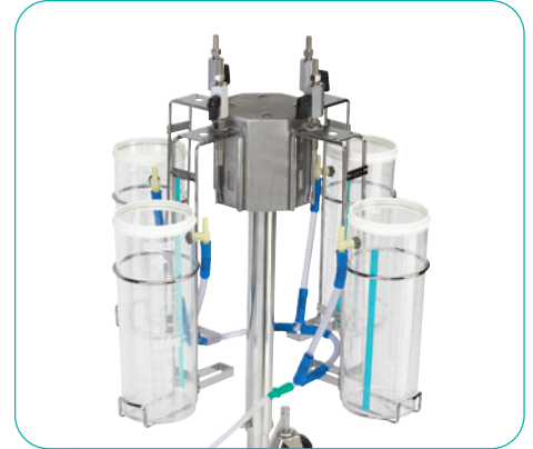
3. Connect tube manifold to vacuum "T"s of each canisters. Connect vacuum source to tube manifold.
