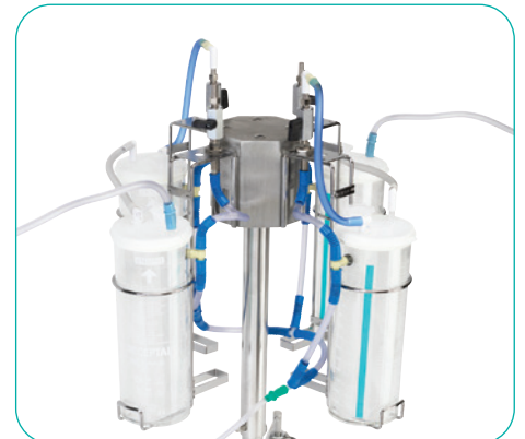
TANDEM CONNECTION SET-UP: Example is for two (2) suctions. Insert same size liners (2 with VAC-GARD® and 2 liners without), secure liner lids to canisters. Connect lid tandem tubing (clear) to patient port of the lid with blue tubing, and switch OFF the valves of liners with clear tube. Connect blue tubing to ON-OFF valve of respective canister. Connect patient tubing to patient port.
