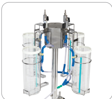
4. Connect vacuum "T"s to ON-OFF valve ports with connecting tube (Item CTM20B). Repeat until all canisters are connected.
