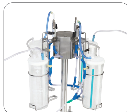
TANDEM CONNECTION SET-UP: Example is for two (2) suction. Insert same size liners (2 with VAC-GARD® and 2 liners without), secure liner lids to canisters. Connect lid tandem tubing (clear) to patient port of the lid with blue tubing, and switch OFF the valves of liners with clear tube. Connect blue tubing to ON-OFF valve of respective canister. Connect patient tubing to patient port.
