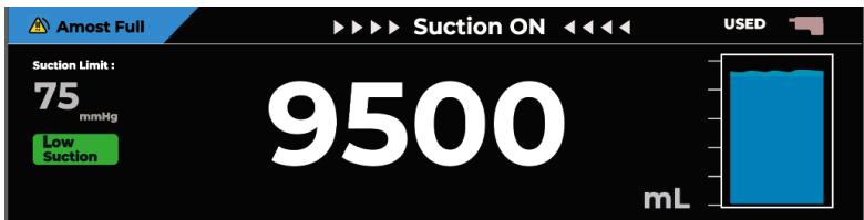
Figure 26 Almost Full Canister Condition (Secondary Control Panel Display)
