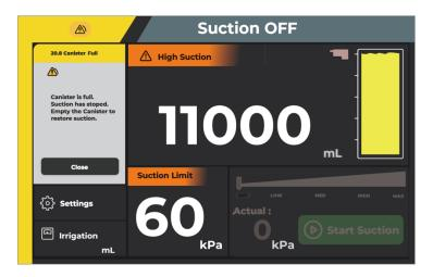
Figure 27 Full Canister Condition (Main Control Panel Display)
